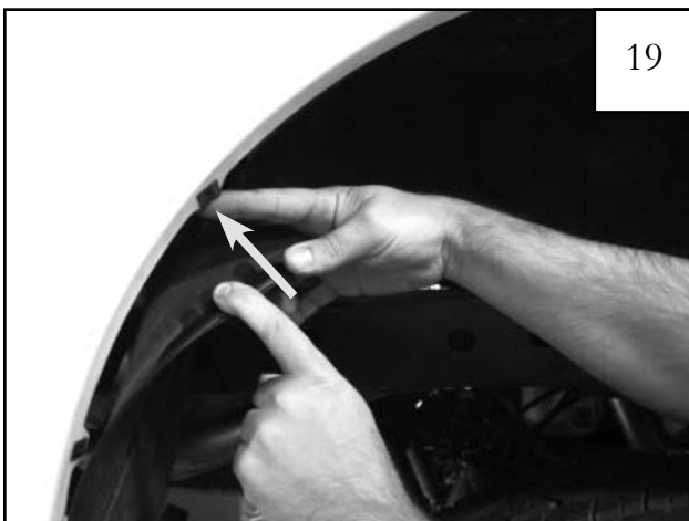
Peel back the rear wheel well liner and install one (1) supplied clip (CL1-0022) at the location indicated. Replace liner to original position.
