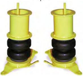
Shock Absorber Relocater kits are mandatory whenever installing and airkit that came with the shocks inside of the Coil Spring.
