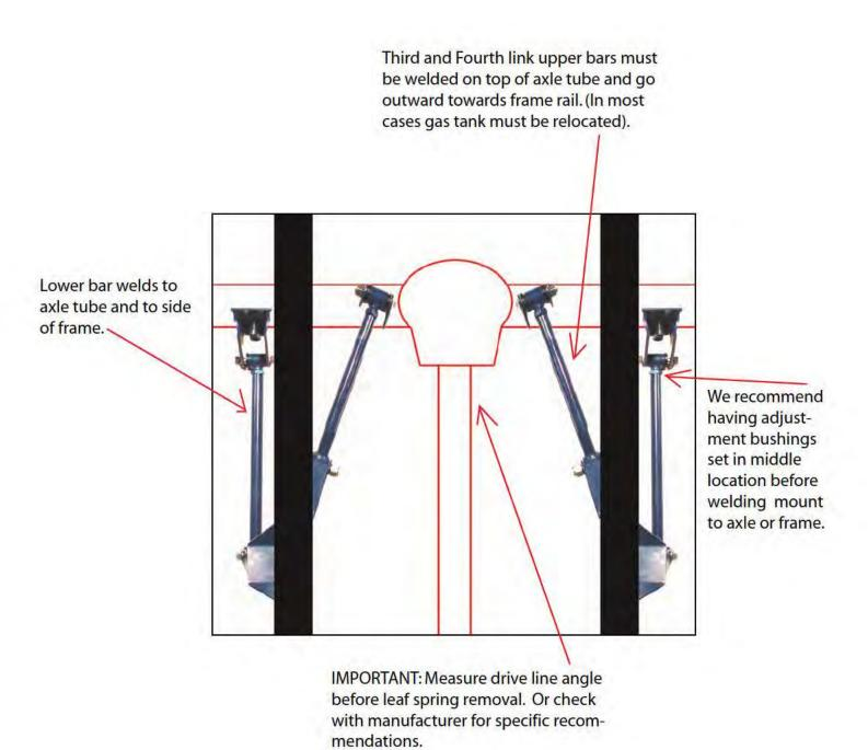
Caution: We recommend tack welding link bars in place and moving vehicle up and down to ensure nothing binds before permanently welding 4 link in place.
