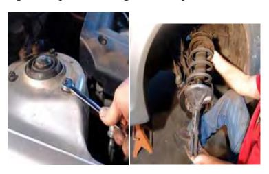
Remove Factory Strut. In most cases, you will reinstall the top bearing plates shown below.
