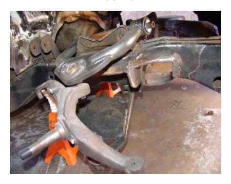
Passenger side with control arms installed and spindle turned to the right. Passenger side with control arms installed and spindle turned to the left. If you are installing Optional Spring Pocket Eliminators,
