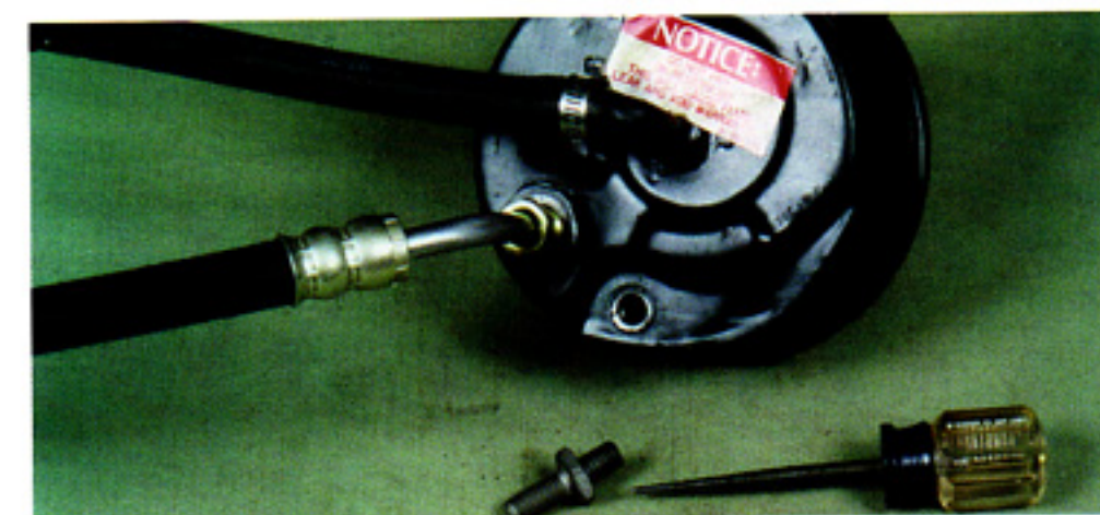
Photo #12: Step 10. Each of the pump brackets has an offset to accommodate the mounting studs on the back of original pumps. Original pumps used special studs (P/N 561350) at the upper and lower locations on the rear of the pump.
