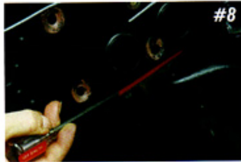
Photos #7 & #8: Step 7. If your car has an original front sway bar, spacers are required to drop the sway bar about 1/8". A spacer will be installed at each frame rail between the sway bar bracket and the frame. From experience, here is a very good way of removing the two bolts securing each of the sway bar brackets. Use a 1/2" short socket on a 1/4" drive ratchet to hold the heads of the two 5/16-18 bolts. These are accessible through two large holes in the outside of the frame. Use 1/2" wrench or socket to remove the nut. After removing the two bolts, position the spacer and secure with the same two bolts. Repeat this procedure for the other side of the sway bar.
