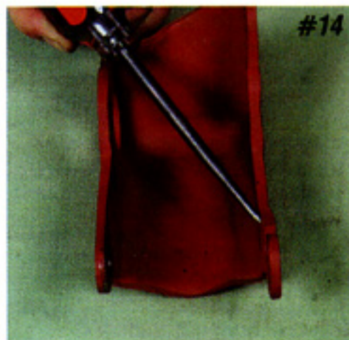
Photos #13 & #14: The forward bracket has an offset at the rear slot and the rear bracket has one at the upper (belt adjusting) location. The replacement pumps do not have the special studs as a result; you must do one of two things to install the pump. The two choices are explained in the next step.
