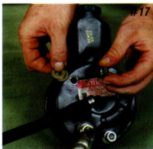
Photos #17 & #18: Step 12. The upper rear location hardware is a 3/8-16 x 3/4" bolt and lock washer with two flat washers used as spacers between the pump and rear bracket (Photo #18). The lower forward location hardware is a 3/8-16 x 1" bolt, flat washer, and lock washer (Photo 19).
