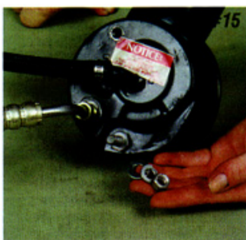
Photos #15 & #16: Step 11. With two studs like original, the pump is very difficult to install. Using just one stud in the lower position makes the installation the easiest. So using one of the special studs is best. Use it in the lower rear position. The hardware required to finish the lower rear location is a flat washer, lock washer, and nut. If you do not use a stud in the lower rear position, two flat washers can be used to take up the space of the stud. The hardware required to finish the lower rear location is a 3/8-16 x 3/4" bolt, flat washer, and lock washer. (In Photo 16; the awl points to the location of the bracket.)
