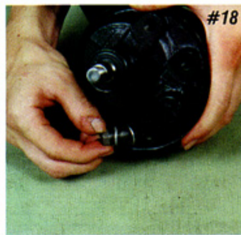
Photos #17 & #18: Step 12. The upper rear location hardware is a 3/8-16 x 3/4" bolt and lock washer with two flat washers used as spacers between the pump and rear bracket (Photo #18). The lower forward location hardware is a 3/8-16 x 1" bolt, flat washer, and lock washer (Photo 19).
