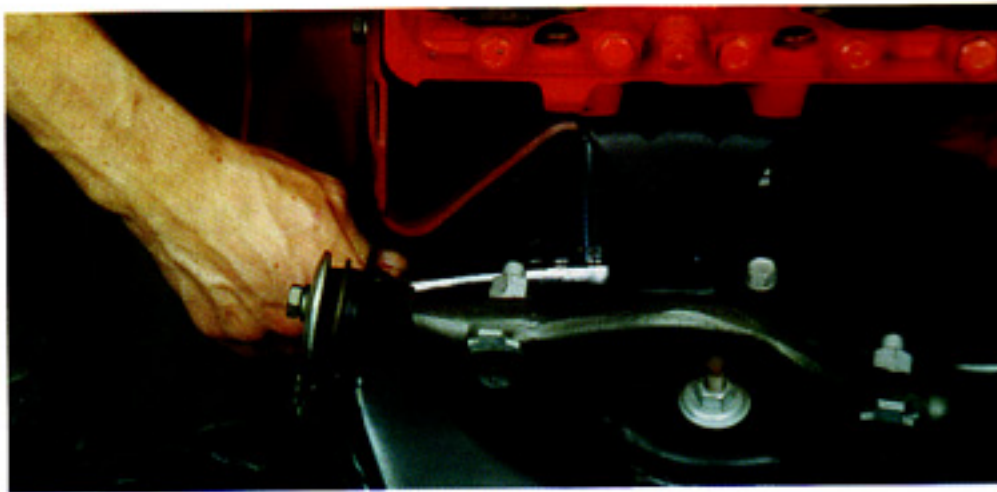
Photo #6: Do not tighten at this time. Install the 7/8" bolt with lock washer through the rear hole in the rear pump bracket, through the motor mount, and then into the block. Now tighten all three bolts, which secure the pump brackets.
