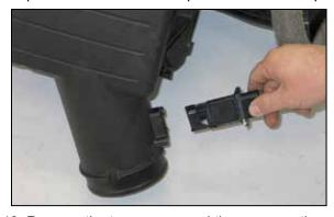
18. Remove the two screws and then remove the mass air sensor from the factory air box.
