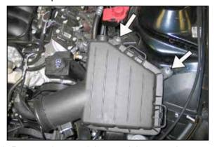
8. Remove the two air box retaining nuts shown.
