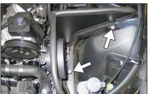
15. Install the heat shield assembly into the vehicle so the inserted nut goes into the air box mounting grommet hole and the tab goes onto the air box mounting stud. Secure the heat shield with the provided hardware.
