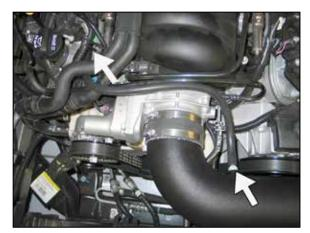
24. Attach the provided crank case vent hose to the 1/4" NPT fitting and then attach the open end to the vent port on the valve cover.
