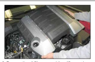
3. Remove the oil filler cap and then lift up and remove the engine cover. Reinstall the oil filler cap. NOTE: On 2014 and later vehicles, the manufacturer changed the crank case vent system. The crank case vent tube will need to be unhooked from the oil filler cap before the cap can be removed from the engine.
