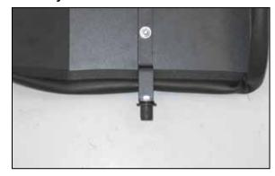
14. Install the inserted nut onto the heat shield mounting bracket using the provided hardware. Do not completely tighten at this time.
