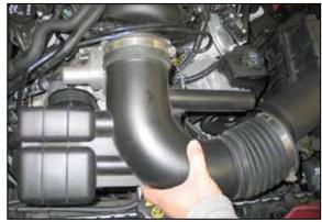
6. Remove the stock intake tube as shown.
