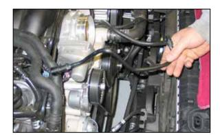
7. Rotate the crank case vent tube 180°, then release the retainer at the valve cover port and then remove the crank case vent tube from the valve cover port.
