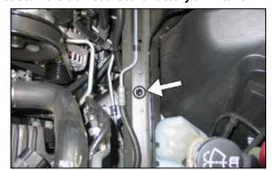
10. Remove the air box mounting grommet shown from the frame rail.
