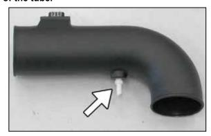
22. Install the provided 1/4 NPT fitting into the K&N® intake tube as shown.
