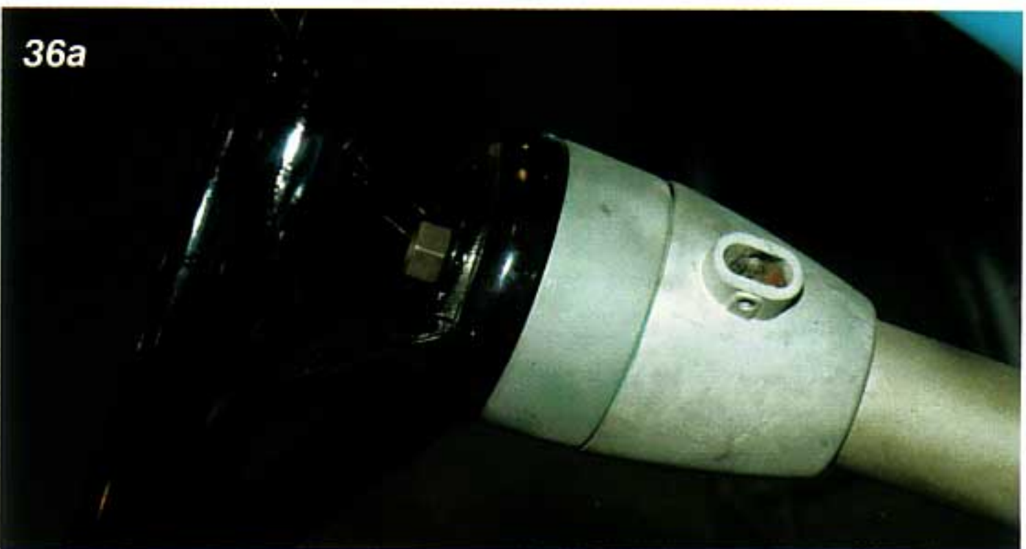
Photo #36a & 36b: Measure the distance between the bottom of the steering wheel and the top of the turn signal housing. We had a measurement of 6-1/2", yours will be different. Remove the shaft from the column. Measure up from the bottom of the steering shaft and cut off the measured amount, which in our case was 6-1/2".
