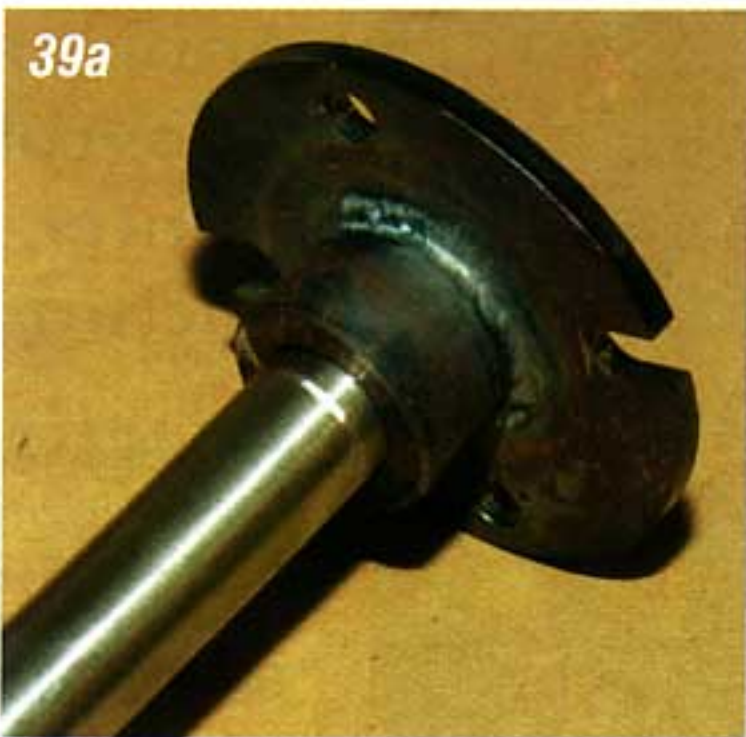
Photo #39a & 39b: Slip the top half of the coupler onto the steering shaft and align with the scribed mark. Weld the coupler to the shaft.
