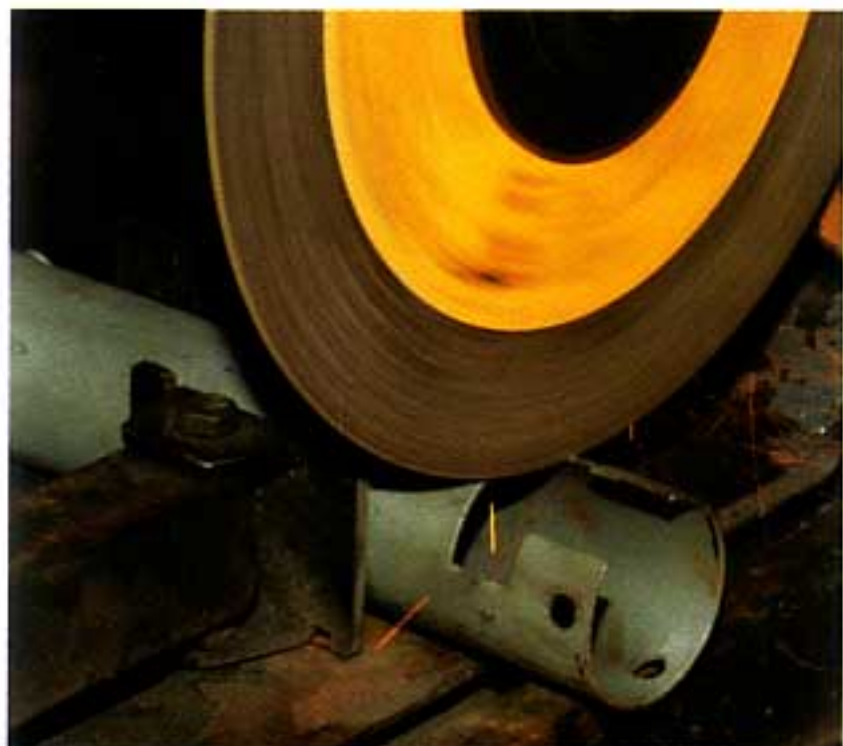
Photo #19: The mast jacket also needs to be shortened. Cut the bottom of the mast jacket off even with the top of the original shift lever opening. This will leave the notch in the mast jacket for the shift detent bracket.
