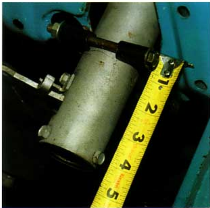
Photo #1: The steering column on a 1955-57 protrudes past the firewall anywhere from 4" to 4 1/2" depending on how the mast jacket (outer column tube) is adjusted at the dash.
