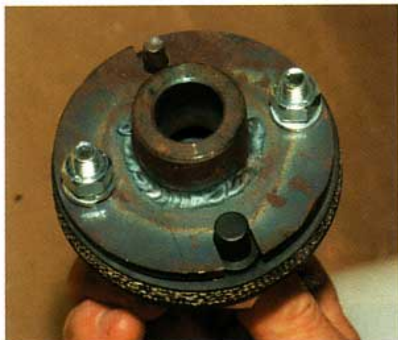
Photo #31: The P/N 53-26 flex coupler has a 3/4"-30 spline on the lower end and a 3/4" smooth bore that must be welded to the original steering shaft that was removed from the stock steering box.
