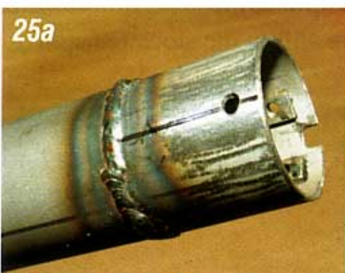
Photo #25a & 25b: Remove the shift tube assembly and measure up 7/16 " from the mark on the bottom of the mast jacket and drill a 3/16 " hole. Reinstall the shift tube assembly and push the aluminum bushing up inside the mast jacket and install the 10-32 machine screw.
