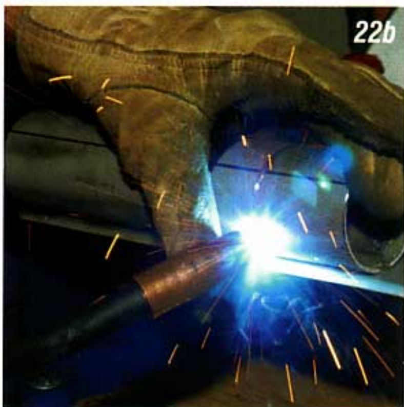
Photo #22a & 22b: Using a piece of angle iron to align the two halves of the mast jacket, orient the two marks and weld together.
