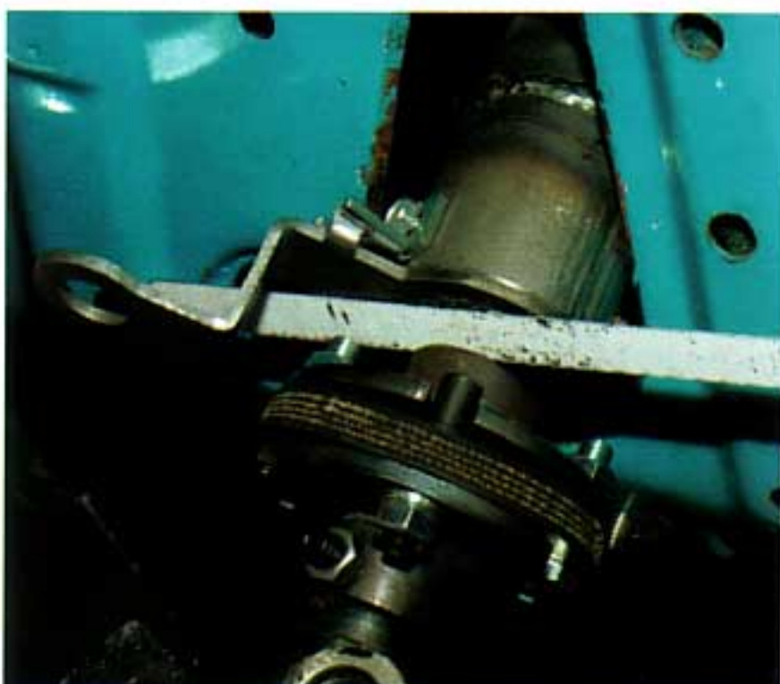
Photo #37: Install the shaft and steering wheel again. Using a hack saw blade, scribe a mark on the shaft at the top of the flex coupler.
