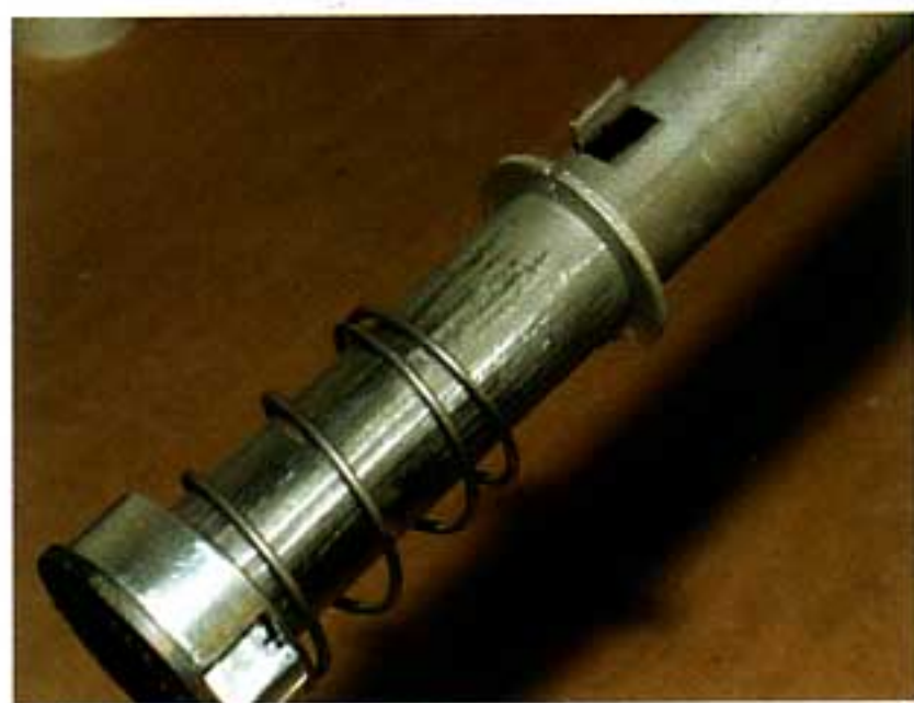
Photo #16: Slide the aluminum bushing all the way down the shift tube. Make certain it will spin freely and not bind on the tube. Measure 15/16" up from the top side of the bushing and mark the tube.
