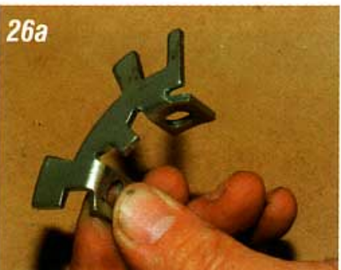
Photo #26a & 26b: The tab on the bottom of the detent bracket fits back into the original notch in the bottom of the mast jacket and into the notch in the aluminum bushing. With the bottom of the mast jacket assembled, you may now reassemble the top of the mast jacket. Be sure the shift tube rotates smoothly in the mast jacket.
