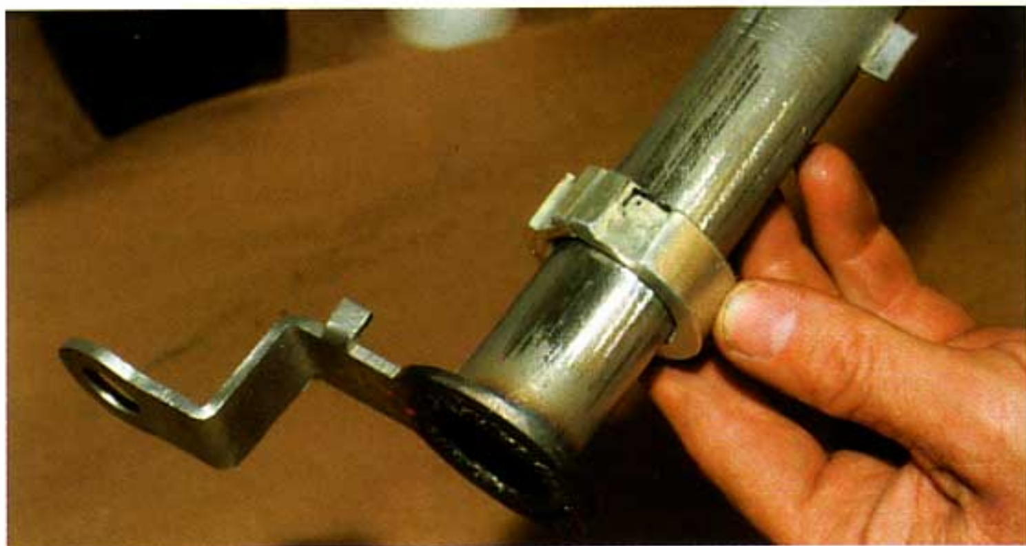
Photo #15: The aluminum bushing has a step and a slot on the inner diameter to allow the bushing to pass by the neutral safety switch tab on the shift tube.
