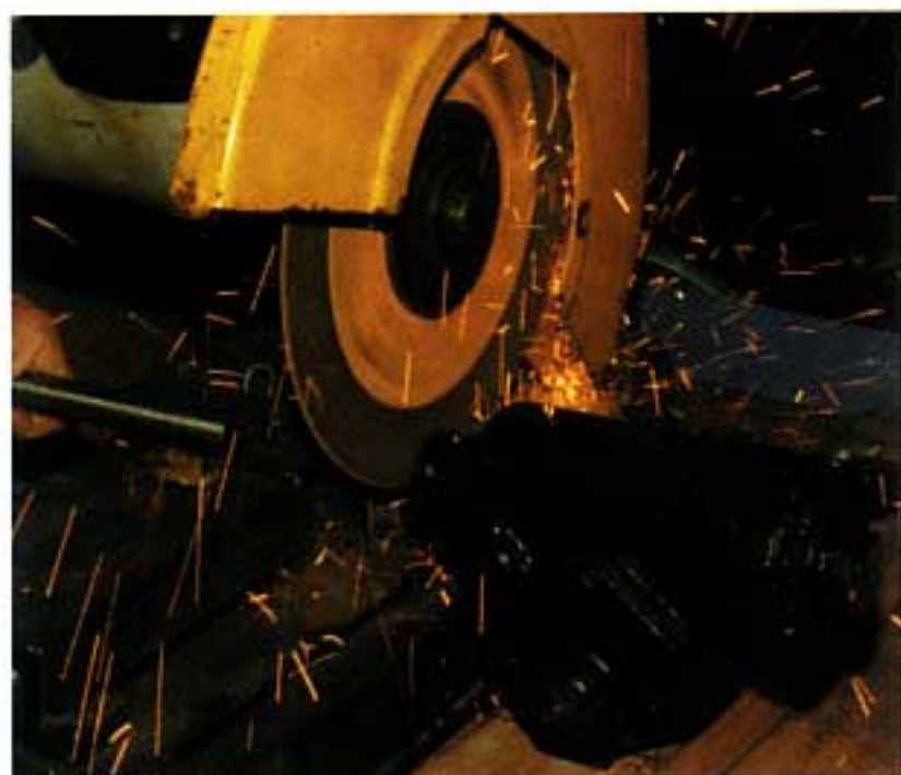
Photo #33: The shaft in the original steering box needs to be cut and removed. This shaft is made of soft steel, so a simple hack saw may be used. We chose to use our chop saw. Cut the shaft flush with the top of the box.
