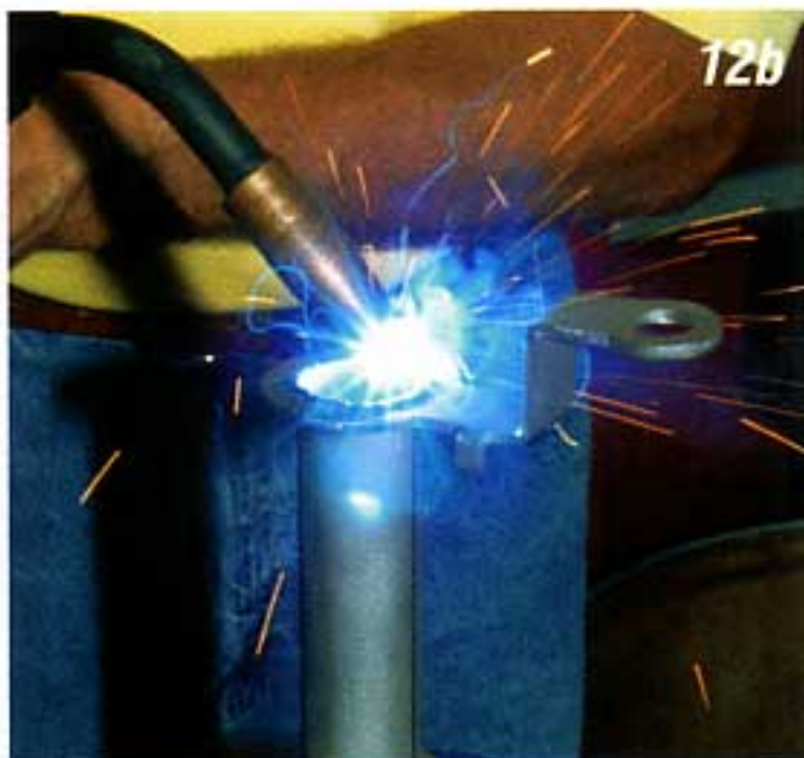
Photo #12a & 12b: The new shift lever included in kit P/N 53-400 has an offset of 1" to clear the firewall. Mark the center of the new shift lever and align the mark with the line on the shift tube. Before welding the new shift lever to the shift tube verify that the overall length of the shift tube is 27-1/4". Weld the bottom side of the shift lever to the very bottom of shift tube.
