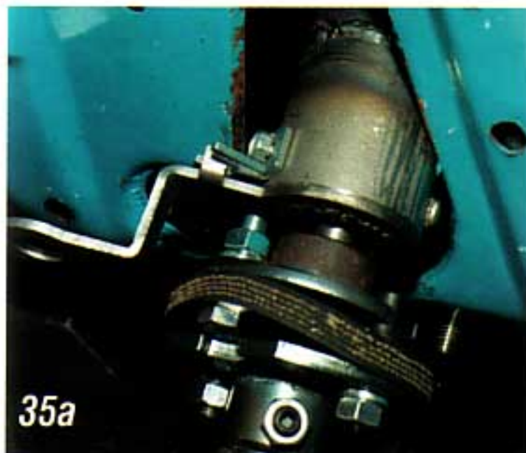
Photo #35a & 35b: Slide the steering shaft down through the column and into the new coupler. The shaft will bottom out against the center pin protruding from the top of the steering box.
