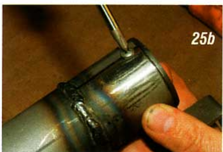
Photo #25a & 25b: Remove the shift tube assembly and measure up 7/16 " from the mark on the bottom of the mast jacket and drill a 3/16 " hole. Reinstall the shift tube assembly and push the aluminum bushing up inside the mast jacket and install the 10-32 machine screw.
