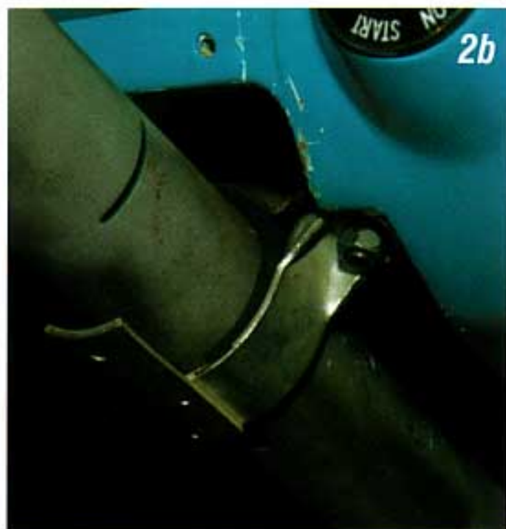
Photo #2a & 2b: The lower part of the mast jacket is held to the firewall with a squeeze clamp bolted to the front side of the firewall in the engine compartment. The upper part of the mast jacket is held to the bottom of the dash on a 1955-56 with a two piece clam shell bracket and a rubber insulator. On 1957 cars there is a bracket that bolts to the bottom of the dash board with two 5/16" bolts and to the mast jacket with two 1/4"-20 bolts. Both types allow the mast jacket to be adjusted up or down to properly adjust the gap between the turn signal housing and the steering wheel.
