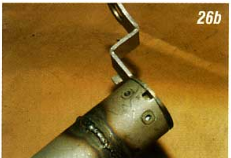
Photo #26a & 26b: The tab on the bottom of the detent bracket fits back into the original notch in the bottom of the mast jacket and into the notch in the aluminum bushing. With the bottom of the mast jacket assembled, you may now reassemble the top of the mast jacket. Be sure the shift tube rotates smoothly in the mast jacket.
