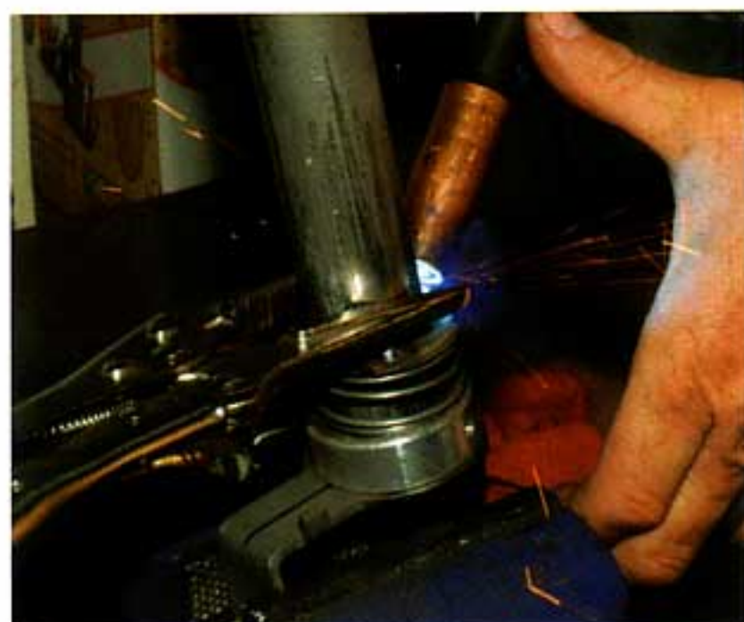
Photo #18: Push the notched washer down to the mark on the shift tube. Using a pair of Vise Grips, hold the washer in place and spot weld it to the tube. Three or four spot welds should be plenty to hold the washer in place.
