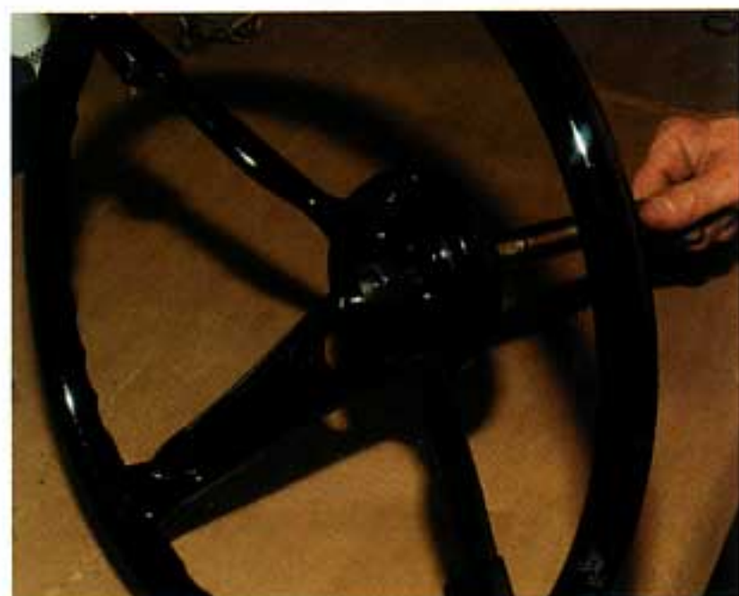
Photo #34: Once the steering shaft is removed, install the steering wheel onto the shaft and tighten the nut.
