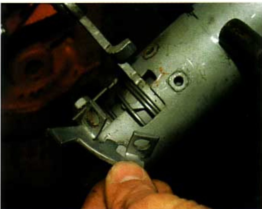
Photo #3: The shift detent bracket bolts to the bottom of the mast jacket with two 1/4"-20 bolts. This bracket must be removed to allow the mast jacket to slip out of the fire wall clamp.
