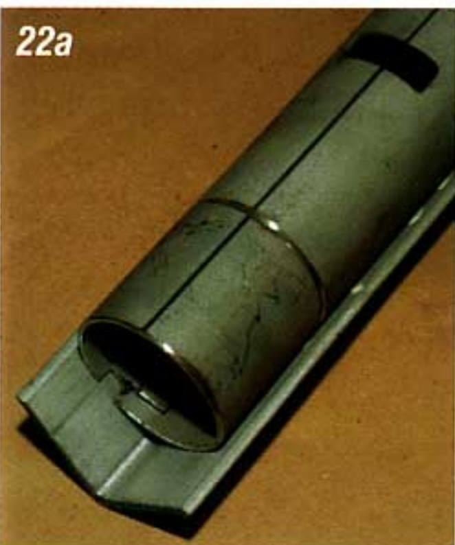
Photo #22a & 22b: Using a piece of angle iron to align the two halves of the mast jacket, orient the two marks and weld together.
