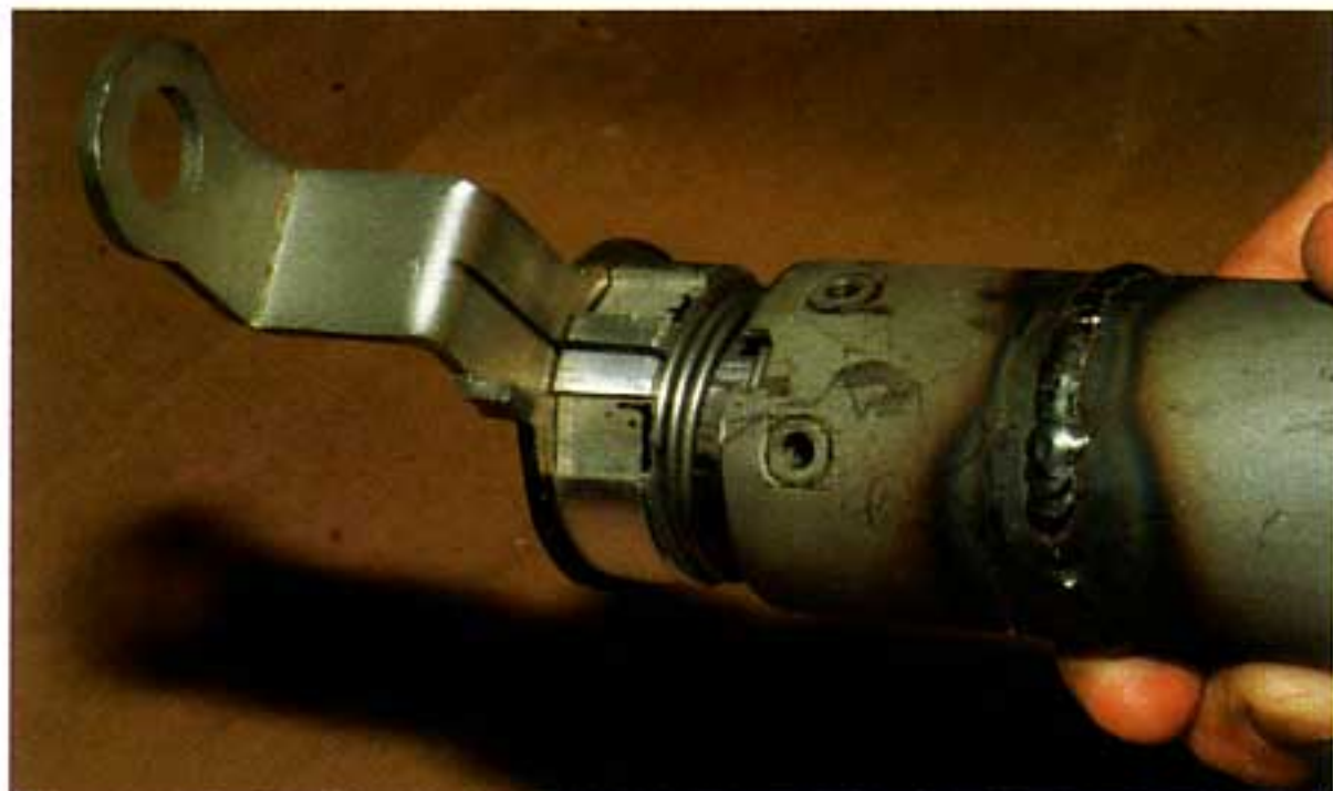
Photo #23: The notches in the steel washer and aluminum bushing will allow the shift tube assembly to bypass the blind nuts in the lower mast jacket.
