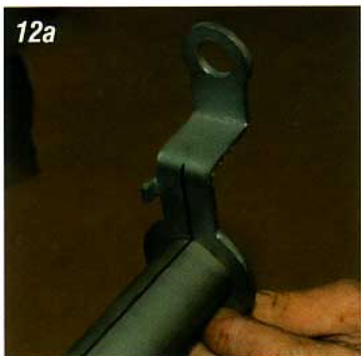
Photo #12a & 12b: The new shift lever included in kit P/N 53-400 has an offset of 1" to clear the firewall. Mark the center of the new shift lever and align the mark with the line on the shift tube. Before welding the new shift lever to the shift tube verify that the overall length of the shift tube is 27-1/4". Weld the bottom side of the shift lever to the very bottom of shift tube.
