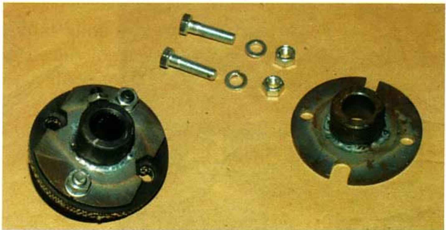
Photo #38: Remove the flex coupler from the steering box and unbolt the top half of the coupler from the fiber center. This will prevent overheating the fiber as the top half of the coupler is welded to the shaft.
