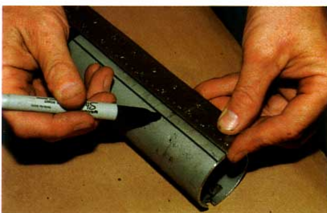
Photo #20: Before making the next cut, make a length-wise line on the mast jacket
