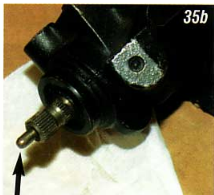
Photo #35a & 35b: Slide the steering shaft down through the column and into the new coupler. The shaft will bottom out against the center pin protruding from the top of the steering box.
