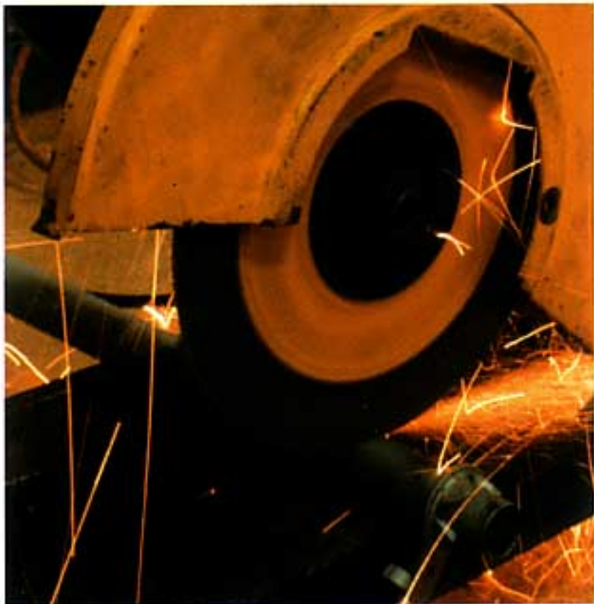
Photo #11: Using a chop saw or band saw cut the shift tube at the mark. It is best not to use a hack saw or hand-held cut-off tool, as a straight cut is important.
