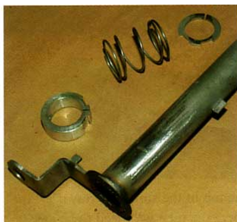
Photo #14: The kit includes an aluminum bushing and steel flat washer to replace the original lower bushing on the modified shift tube. The stock lower spring will be reused.
