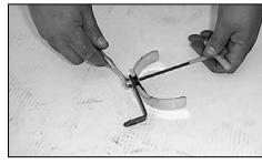
23. Assemble the L bracket and saddle bracket using the hardware provided.
