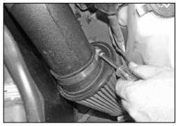
40. Install the air filter element onto the intake tube rotate, for best clearance and secure it with the provided hose clamp.
