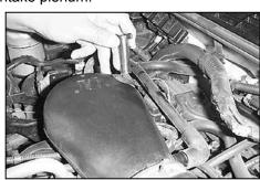
4. Loosen and remove the tall wing nut that retains the intake plenum.
