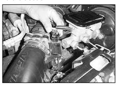
2. Disconnect the mass air sensor and air temp. sensor electrical connections.
