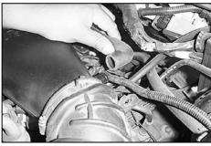
3. Disconnect the crank case vent line from the intake plenum.
