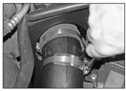
39. Attach the saddle/bracket assembly to the secondary intake tube using the provided hose clamp.
