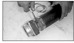
30. Using the hose clamp provided, attach the silicone step hose to the mass air sensor with the directional arrow as shown above.
