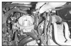
12. Remove the nut that retains the throttle cable bracket.
