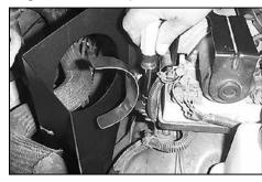
24. Install the saddle/bracket assembly onto the original air box mounting stud and secure with the hardware provided.
