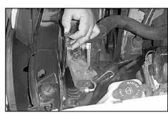
9. Pull the release tab and slide the retainer bracket upward to remove it from the radiator core support.
