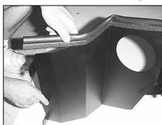
36. Install trim seal onto the heat shield.
