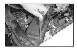
5. Loosen the four screws that retain the air box top to the air box base.
