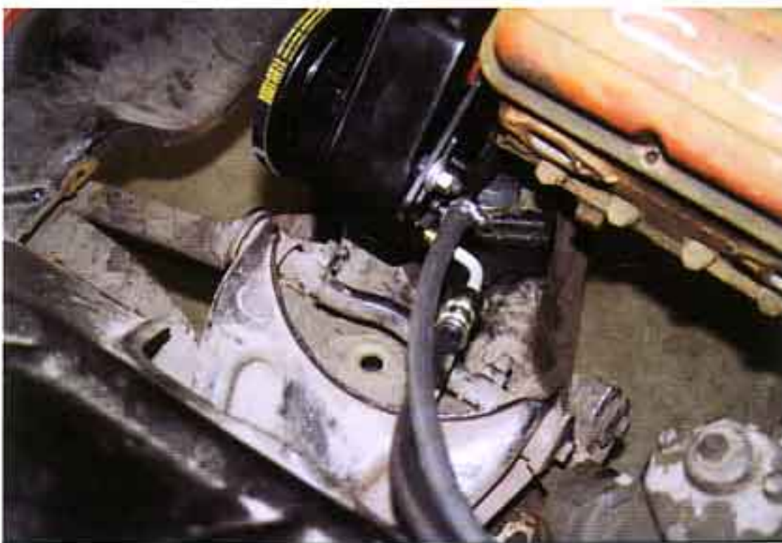
Photo #7: The pressure hose has a 90 degree fitting on the end that screws directly into the large
