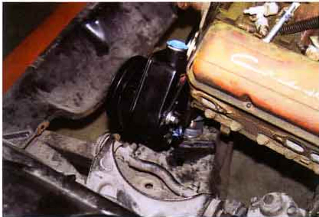
Photo #4: The adjusting arm for the power steering pump attaches to the upper water pump
