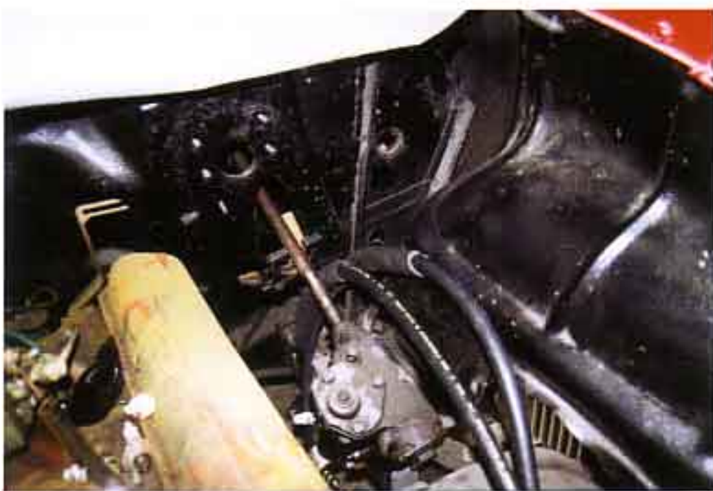
Photo #6: Route the two hoses to the outside of the steering shaft. Both hoses have the foam rubber covering just like the factory hoses.
