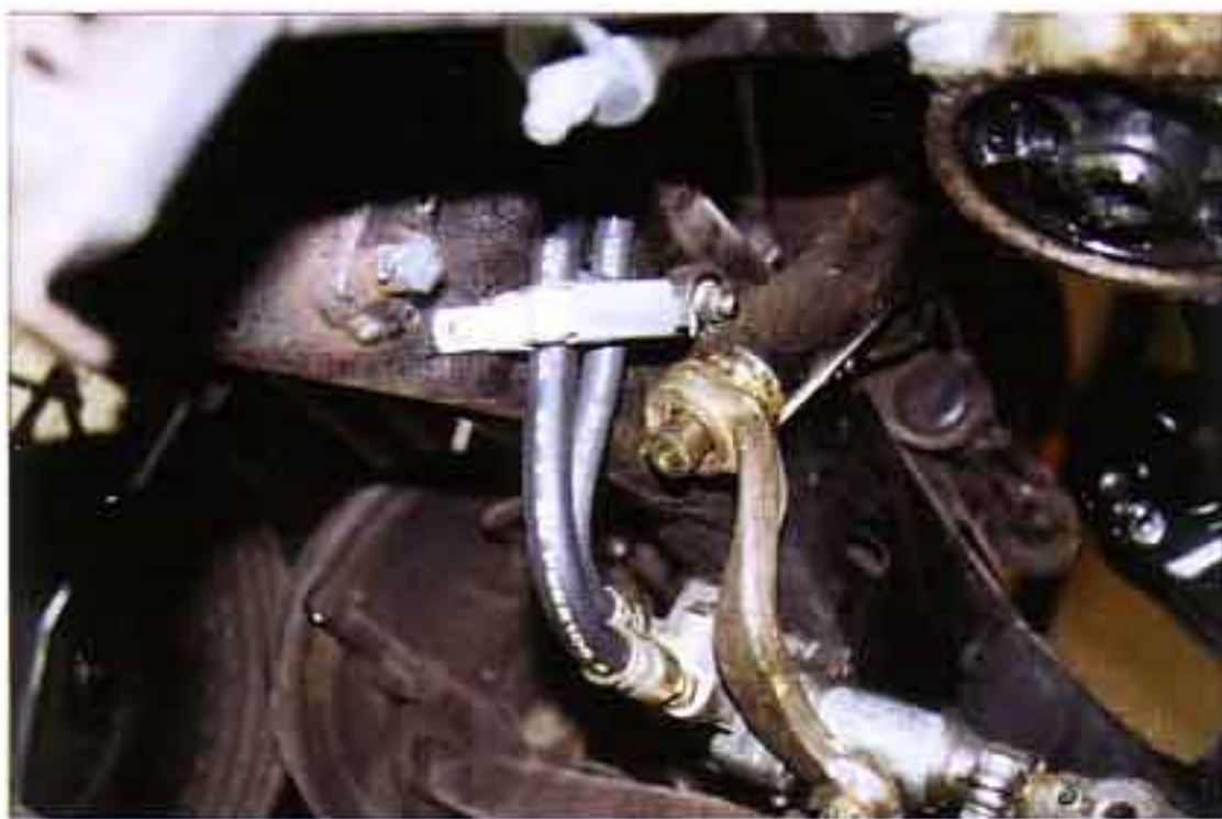
Photo #5: The pressure and return hoses attach to the end of the control valve and are routed up
