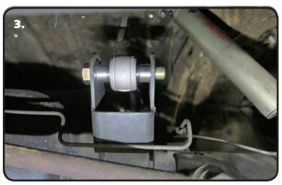
**3.** Install a 5/8" flat washer on a 5/8"-18 x 3 3/4" hex bolt through the mount and control arm R-Joint. Install a 5/8" flat washer, followed by a 5/8"-18 nylok jam nut onto the threads of the bolt. Tighten the hardware enough to eliminate any gaps.
