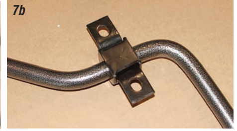
Photos 7a & 7b: The D-shape bushings are split and install on the rear part of the anti-sway bar that is parallel with the rear end housing. The steel U-bracket wraps around the D-bushing and holds the anti-sway bar to the rear end mounting brackets.
