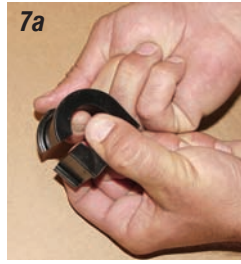
Photos 7a & 7b: The D-shape bushings are split and install on the rear part of the anti-sway bar that is parallel with the rear end housing. The steel U-bracket wraps around the D-bushing and holds the anti-sway bar to the rear end mounting brackets.
