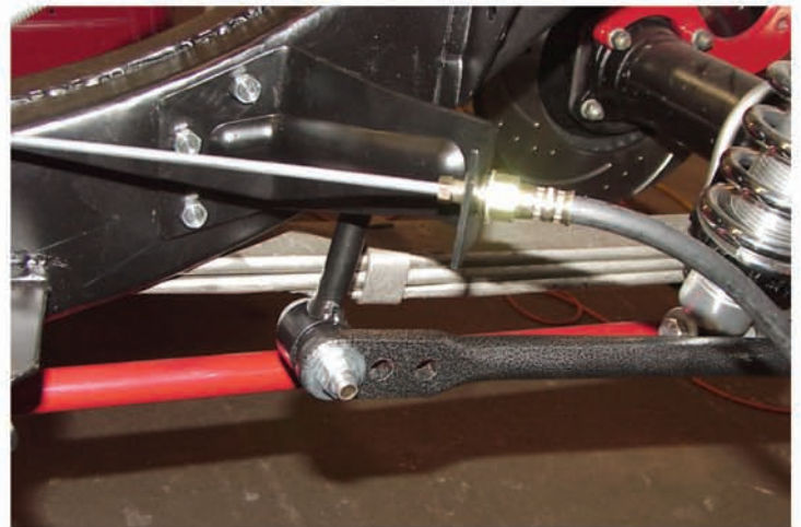
Photo 20: Hellwig recommends installing the end links in the forward-most holes of the anti-sway bar for the first couple of test drives. The forward hole in the anti-sway bar will give you the softest ride, the center will be firmer and the rear hole will be for the firmest ride. Once you drive the car and desire firmer, more stable cornering, adjust to the rear holes until you get the handling you desire. ✓
