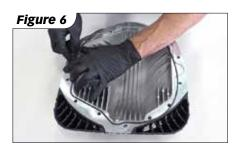
**7.** Install the Banks cover and re-attach brackets to the cover using included M8 bolts. Apply small amount of threadblocker on the bolts. Torque the bolts to 12 lb/ft (29 N.m) using a 10mm 12 pt socket.
