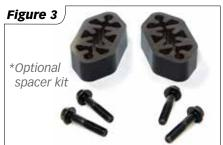
Note: RAM trucks equipped with a rear sway bar require the installation of a \*spacer kit (PN19249-2) to provide proper clearance between the sway bar and the differential cover.
