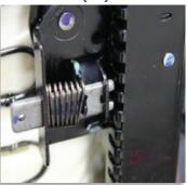
(2A) You can now attach the fixed mounts if applicable to your floor pan. Use your O.E.M. hardware to mount your adapters to the floor boards
