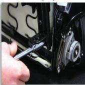
Attach return spring as shown in illustration (2A), (2B) between the two sprung points. This will allow the seats locking mechanism to activate once the seat is slid to the desired position of choice
