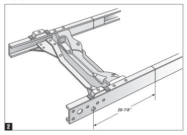
4. When you are happy with the fitment and the crossmember fits square to the frame, mark the spindle centerline on the crossmember (figure 3) making sure that your mark is parallel to your axle centerline you marked on the frame. Next, tack weld the lower crossmember in place.
